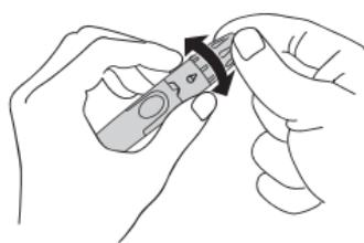
5. Turn the tip until the mark (white drop) points to the requested penetration depth. You can adjust 6 penetration depths.
